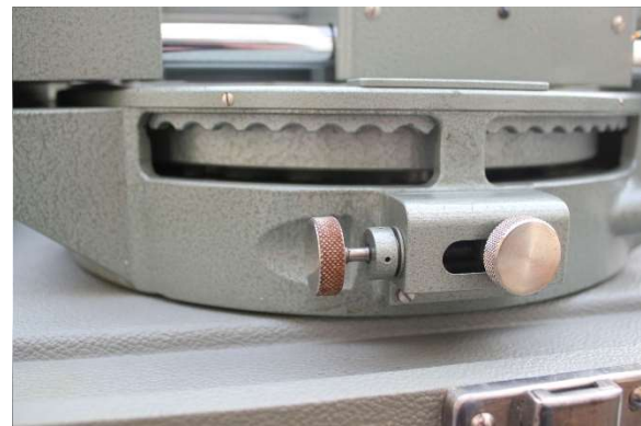
FIGURE 11. Grip Recesses for Turning the Pitch Circle. The Left Setscrew is used for Fine Adjustment, the Right one for Fixing the Pitch Circle.
